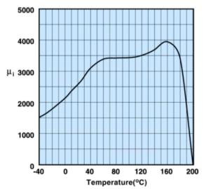
Measured on a 17/10/6mm toroid at 10kHz.
