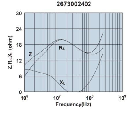
Impedance, reactance, and resistance vs. frequency.
